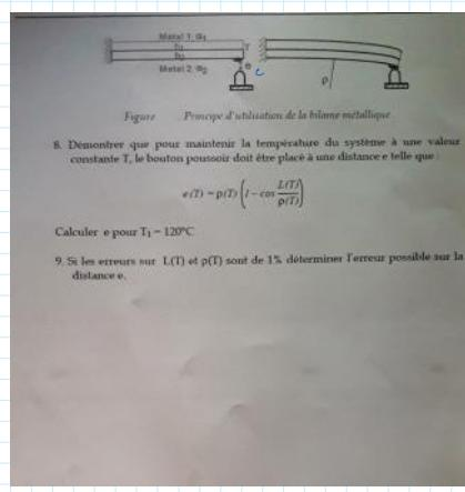
$$\Delta L = \alpha L_0 \Delta T = \alpha l_0 (T - T_0)$$
